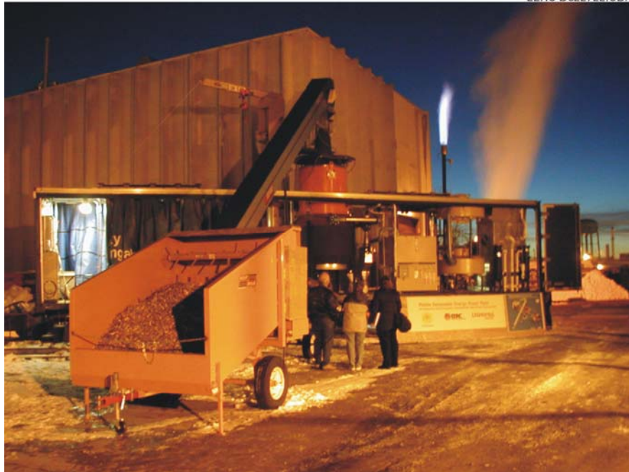
Figure 1. Portable gasification system in operation at the EERC.
