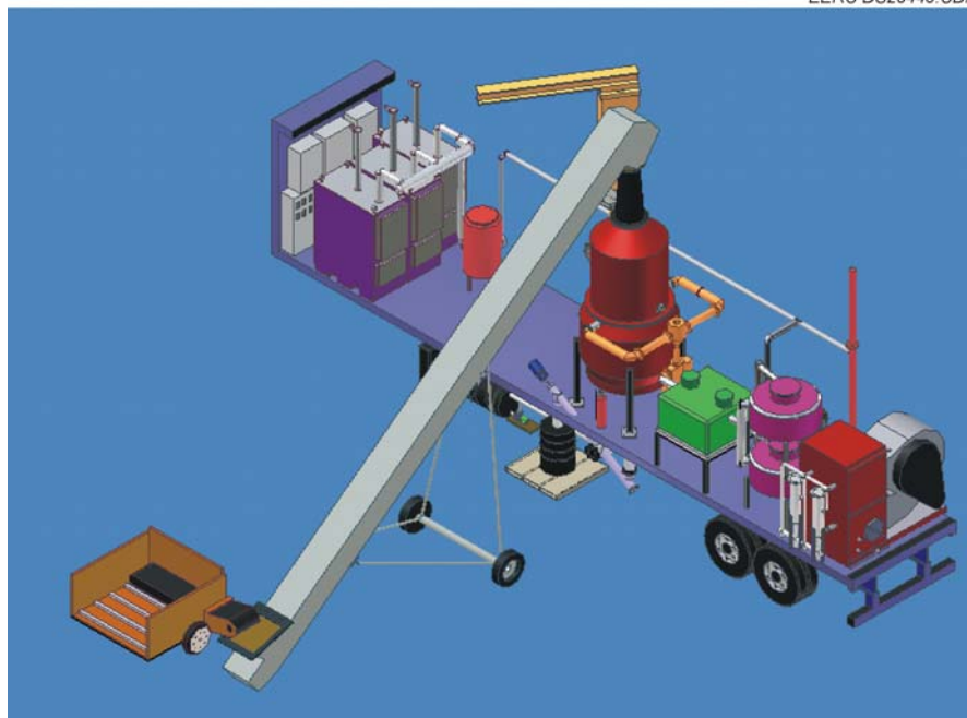
Figure 2. Portable gasification system and fuel.
