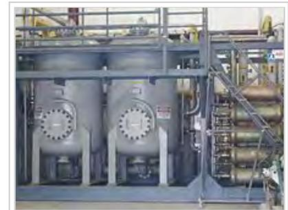
Gas separator membrane skid used in membrane separation process to extract carbon dioxide<sup>[13]</sup>
