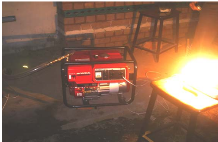
Figure 9 Synthesis Gas Operating the Engine
