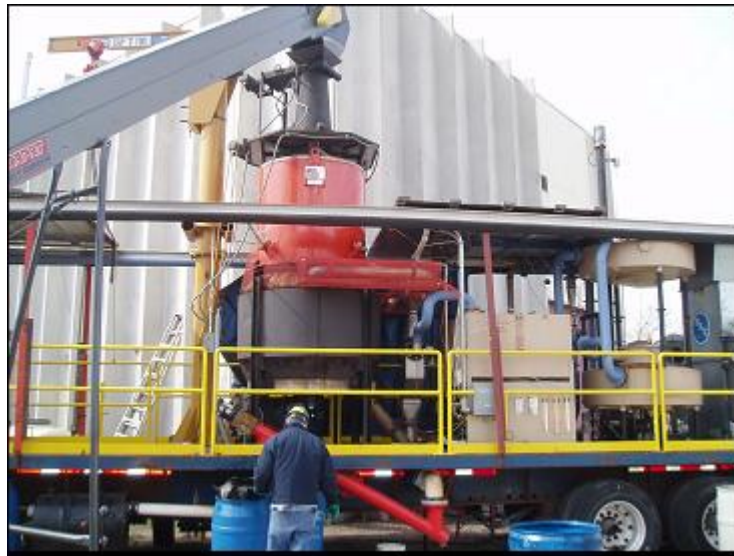
Figure 5: Trailer Mounted 200 kWe Gasifier, FlexEnergy Ltd, 2005
