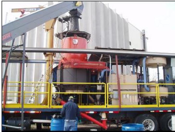
Figure 5: Trailer Mounted 200 kWe Gasifier, FlexEnergy Ltd, 2005
