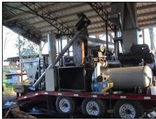
Figure 9: 5 TPD Bio-Oil Pilot Plant (Renewable Oil International)
