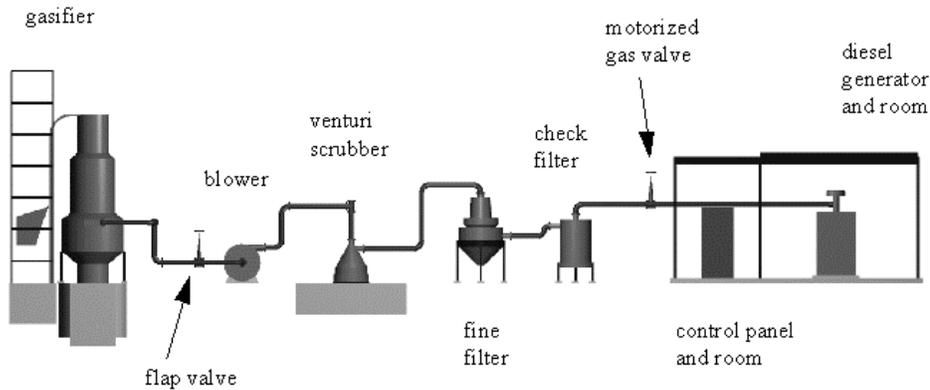
**Figure 2 – Downdraft Gasification System**
