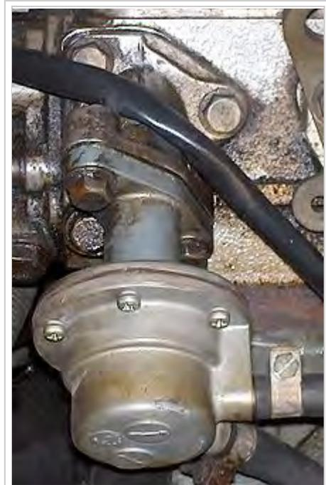
Mechanical fuel pump, fitted to cylinder head
