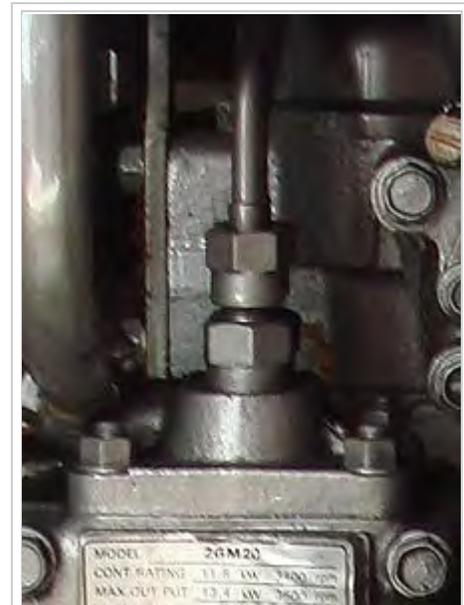
A high-pressure fuel pump on a Yanmar 2GM20 marine diesel engine.
