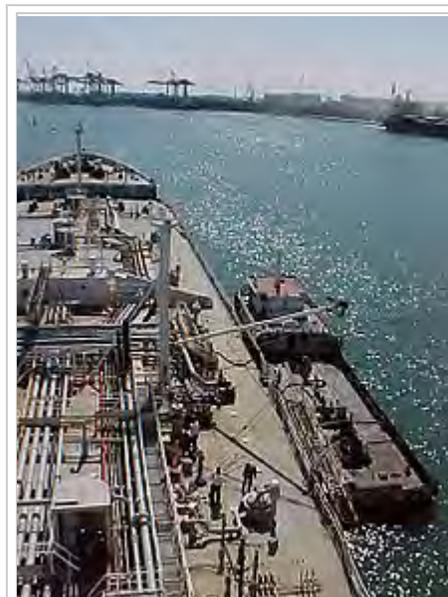
an oil tanker taking on fuel, or "bunkering."
