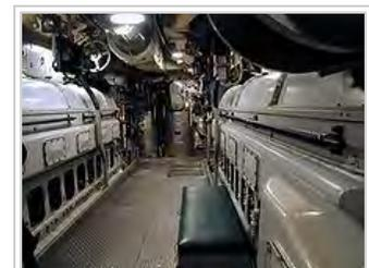
Fairbanks-Morse opposed piston diesel engines on a submarine
