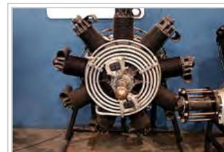
Packard DR-980 9-cylinder diesel aircraft engine
