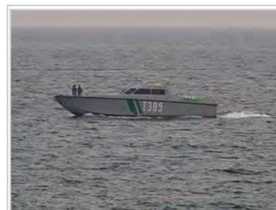
Bio Diesel Powered Fast Attack Craft Of Indian Navy patrolling during IFR 2016. The green bands on the vessels are indicative of the fact that the vessels are powered by bio-diesel
