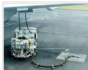
At some airports, underground fuel pipes allow refueling without the need for tank trucks. Trucks just carry the necessary hoses and pressure apparatus, but no fuel.
