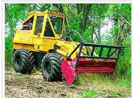
Hydraulic-powered mulching attachment on rubber-tired tractor
