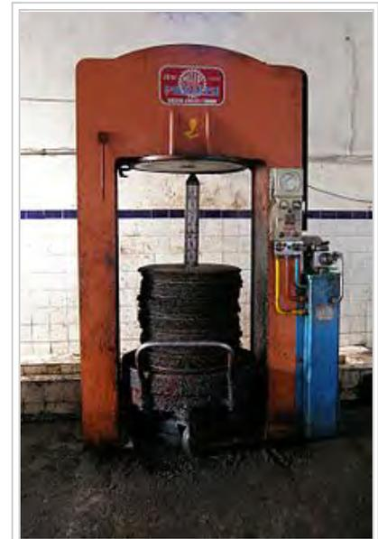
Press with stack of fiber disks
