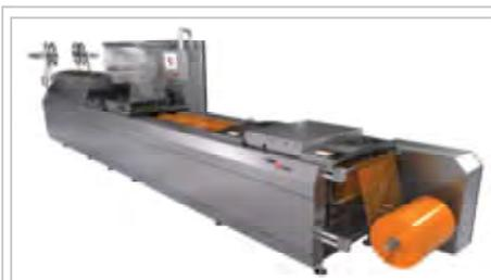
Thermoform packaging machines are used in larger production facilities for vacuum packaging products.
