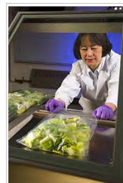
Package testing: Heat sealing film for evaluation of shelf life of lettuce
