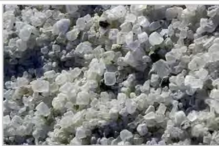
Picture of solid form of rock salt used for ice removal on streets.
