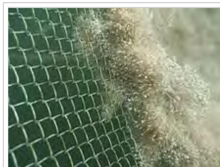
There is no biofouling on a copper alloy mesh after 4 months immersed in the waters of the North Atlantic (foreground), whereas hydroids have grown on high-density polyethylene tubing (background).
