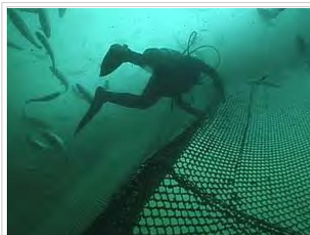
A copper alloy pen that has been deployed on a fish farm at depth of 14 feet for one year shows no signs of biofouling.
