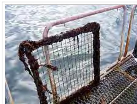
Section of a fish net on a salmon farm near Puerto Montt, Chile. The copper alloy woven mesh inside the frame has resisted biofouling whereas PVC (i.e., the frame around the mesh) is heavily fouled.
