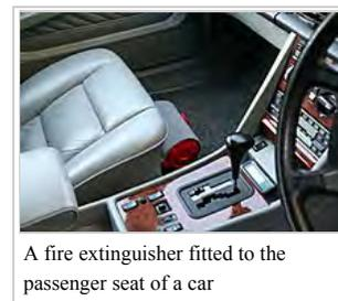
A fire extinguisher fitted to the passenger seat of a car
