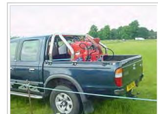
Heavy-duty CO<sub>2</sub>-powered fire extinguisher on standby at a temporary helicopter landing site
