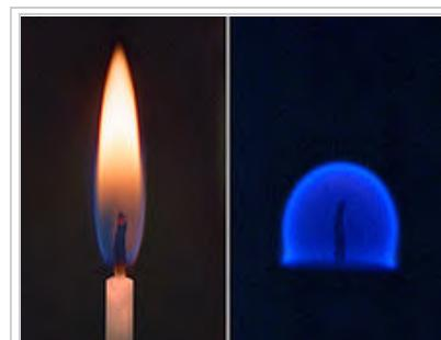
Fire is affected by gravity. Left: Flame on Earth; Right: Flame on ISS
