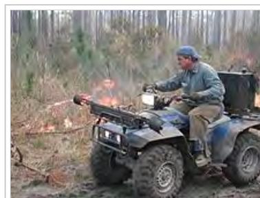
Firing the woods in a South Carolina forest with a custom made driptorch mounted on an ATV. The device spits flaming fuel oil from the side, instantly igniting the leaf litter.
