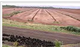
Industrial milled peat production in a section of the Bog of Allen in the Irish Midlands: The 'turf' in the foreground is machine-produced for domestic use.
