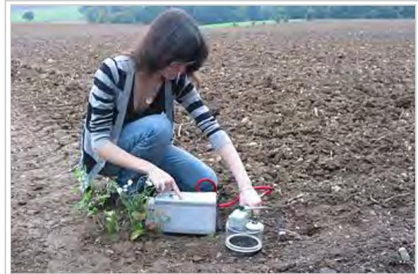
A portable soil respiration system measuring soil CO<sub>2</sub> flux
