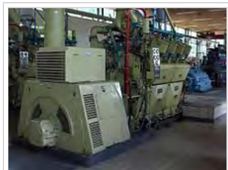
Brons two-stroke V8 Diesel engine driving a N.V. Heemaf generator.
