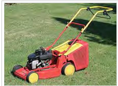
Rotary lawn mower, with a vertical shaft engine
