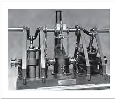
Model of a Maudslay oscillating engine
