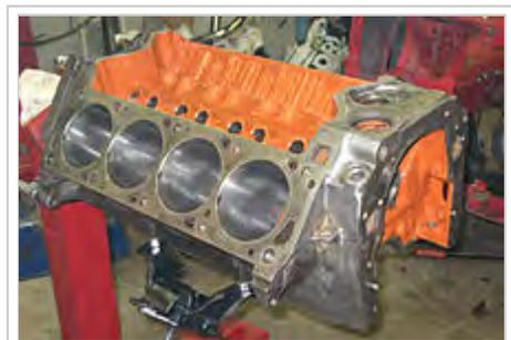
Bare cylinder block of a V8 engine
