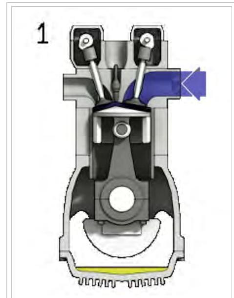
Four-stroke cycle used in gasoline/petrol engines. **1** = Intake, **2** = Compression, **3** = Power, **4** = Exhaust. The right blue side is the intake port and the left brown side is the exhaust port. The cylinder wall is a thin sleeve surrounding the piston head which creates a space for the combustion of fuel and the genesis of mechanical energy.
