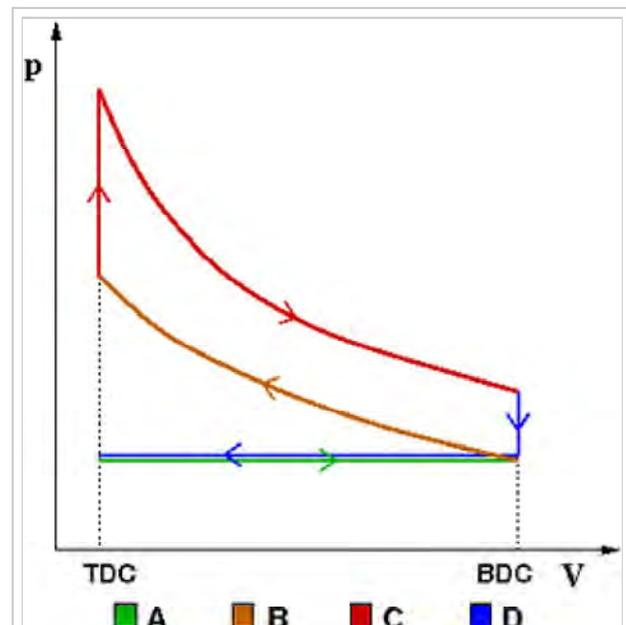
The idealized four-stroke Otto cycle p-V diagram: the intake (A) stroke is performed by an isobaric expansion, followed by the compression (B) stroke, performed by an adiabatic compression. Through the combustion of fuel an isochoric process is produced, followed by an adiabatic expansion, characterizing the power (C) stroke. The cycle is closed by an isochoric process and an isobaric compression, characterizing the exhaust (D) stroke.
