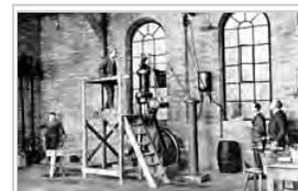
Diesel's prototype engine
