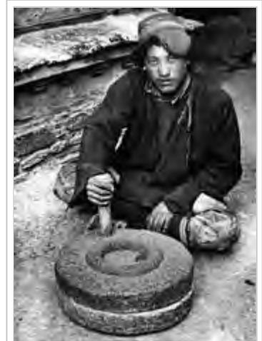
Tibetan operating a quern (1938). The upright handle of such rotary handmills, set at a distance from the centre of rotation, works as a crank.<sup>[3][4]</sup>
