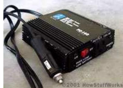
From this discussion you can see that an inverter only makes sense for very small power loads over relatively short time frames. You can build a large and elaborate battery system to run your inverter if you choose, but that can get expensive.
