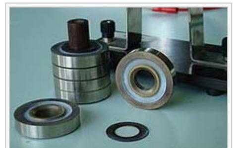
The parts of the spark gap
