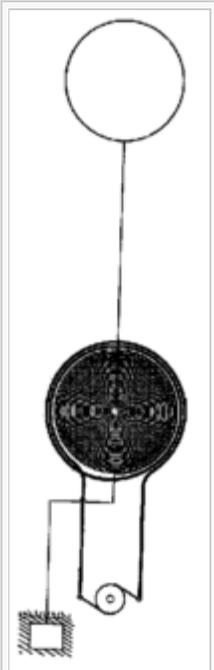
Tesla coil transformer wound in the form of a flat spiral. This is the transmitter form as
