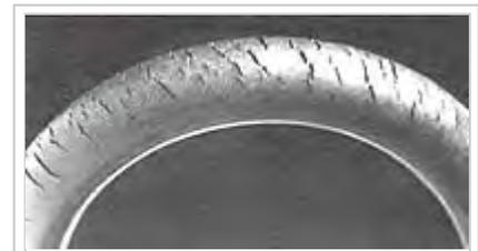
Ozone cracking in natural rubber tubing
