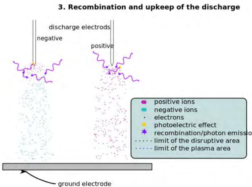
5. At a certain distance from the electrode, the electric field becomes low enough that it no longer imparts enough energy to the electrons to ionize atoms when they collide. This is the outer edge of the corona. Outside this the ions move through the air without creating new ions. The outward moving ions are attracted to the opposite electrode and eventually reach it and combine with electrons from the electrode to become neutral atoms again, completing the circuit.
