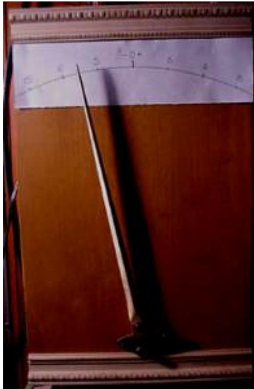
The meter consists of a wooden back, a long wooden needle(14" long), which pivots on a nail. To the bottom of the long wooden needle is a surplus computer hard drive magnet glued on with super-glue. You can get the magnet out of most computer hard drives, or...we sell them, between \$1 and \$12, depending upon the scale of meter you have in mind. (it would be great to make a BIG one)
