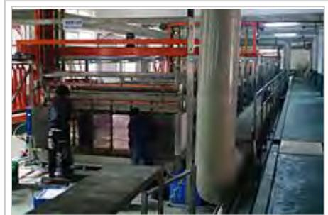
Copper electroplating machine for layering PCBs
