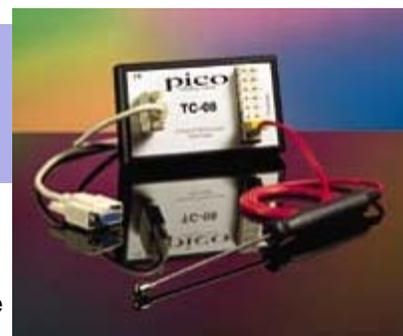
Pico has two products designed to allow temperature to be measured and recorded using thermocouples. The [TC-08](#) interfaces up to 8 thermocouples of any type to a PC. The [CM005](#) K Type thermocouple signal conditioner provides a simple way of connecting a thermocouple to the ADC16 data logger, the Enviromon network or any of our PC based oscilloscopes.
