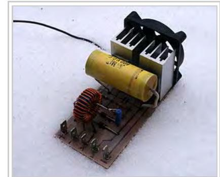
Zero voltage switched mode power supplies require only small heatsinks as little energy is lost as heat. This allows them to be small. This ZVS can deliver more than 1 kilowatt. Transformer is not shown.
