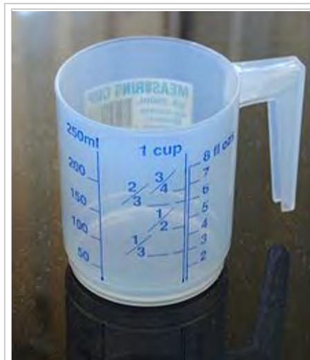
A measuring cup can be used to measure volumes of liquids. This cup measures volume in units of cups, fluid ounces, and millilitres.
