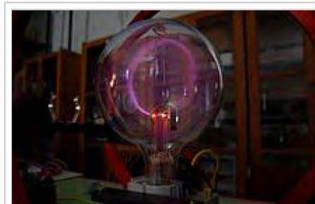
A beam of electrons deflected in a circle by a magnetic field<sup>[27]</sup>
