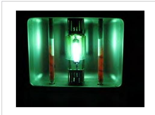
The deep violet glow of a mercury vapor discharge in a germicidal lamp, whose spectrum is rich in invisible ultraviolet radiation.
