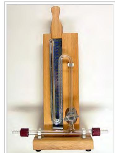
Mercury manometer to measure pressure
