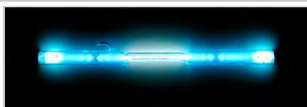
Mercury-discharge spectral calibration lamp
