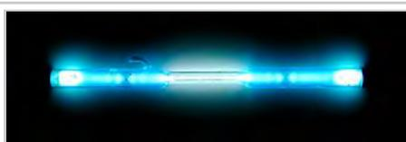
Mercury-discharge spectral calibration lamp
