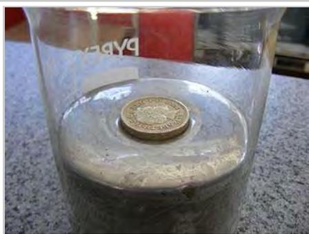
A pound coin (density  $\sim 7.6\text{ g/cm}^3$ ) floats in mercury due to the combination of the buoyant force and surface tension.
