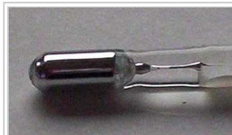
The bulb of a mercury-in-glass thermometer
