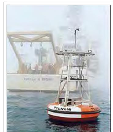
One of the deep water buoys used in the DART tsunami warning system
