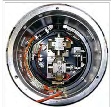
A low-frequency 3-direction ocean-bottom seismometer (cover removed). Two masses for x- and y-direction can be seen, the third one for z-direction is below. This model is a CMG-40TOBS, manufactured by Gralp Systems Ltd and is part of the Monterey Accelerated Research System (<http://www.mbari.org/mars/default.htm>)
