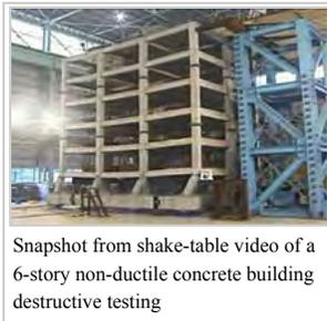
**Seismic performance assessment** or seismic structural analysis is a powerful tool of earthquake engineering which utilizes detailed modelling of the structure together with methods of structural analysis to gain a better understanding of seismic performance of building and non-building structures. The technique as a formal concept is a relatively recent development.
