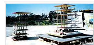
Concurrent experiments with two building models which are kinematically equivalent to a real prototype.<sup>[19]</sup>
