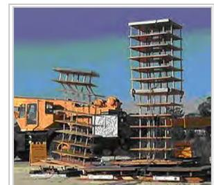
Shake-table crash testing of a regular building model (left) and a base-isolated building model (right)<sup>[3]</sup> at UCSD
