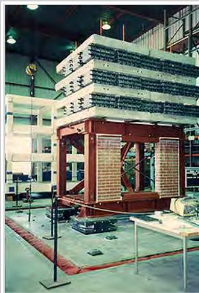
Shake-table testing of Friction Pendulum Bearings at EERC
