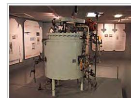
A 1957 fermentor (bioreactor) used to grow *Penicillium* mould.
