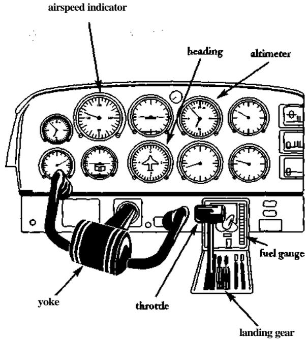
**THROTTLE.** This controls airspeed (power) and also the nose attitude, or its relation to the horizon. It is a lever between the seats and is always black. Pull it toward you to slow the plane and cause it to descend, push it away to speed up the plane and cause it to ascend. The engine will get more or less quiet depending on the direction the throttle is moved.
