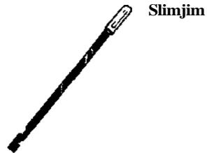
*Slide the Slimjim between the glass and the weather stripping. Feel for the lock rod. Move the tool back and forth gently until the lock flips over.*
