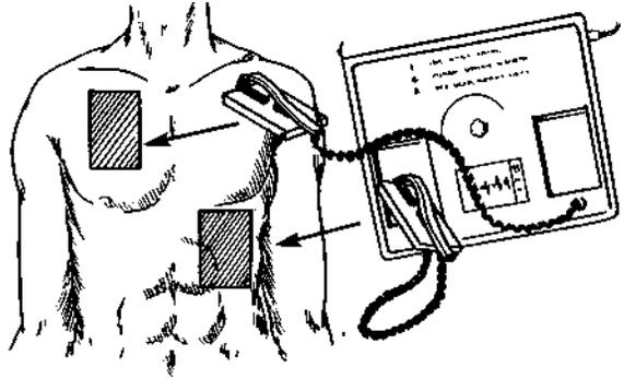
**3 Plug the pads into the connector.**
