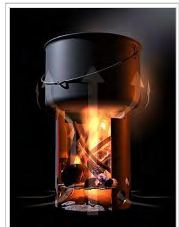
Heat convection in a hobo stove (schematic)
