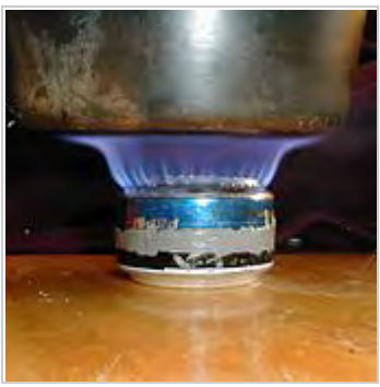
A beverage-can stove, fueled by denatured alcohol (the pot stand is omitted for clarity)
