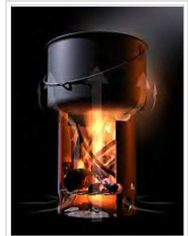
Heat convection in a hobo stove (schematic)
