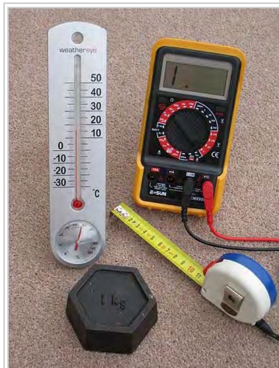
"The metric system is for all people for all time." (Condorcet 1791) Four objects used in making measurements in everyday situations that have metric calibrations are shown: a tape measure calibrated in centimetres, a thermometer calibrated in degrees Celsius, a kilogram mass, and an electrical multimeter which measures volts, amps and ohms.
