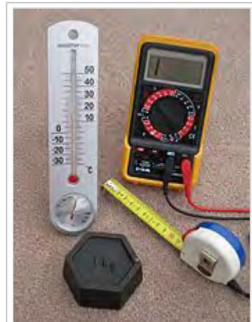
Four measuring devices having metric calibrations
