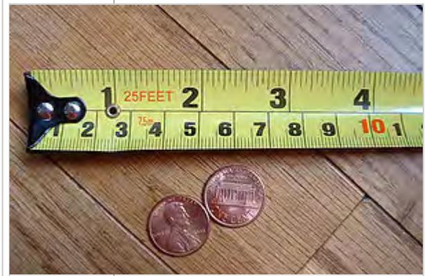
A typical tape measure with both Metric and Imperial units and two US pennies for comparison
