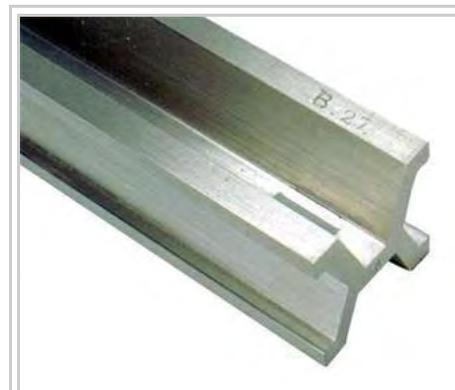
Closeup of the National Prototype Metre, serial number 27, allocated to the United States
