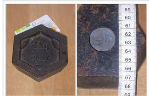
Top view of the 2 kg weight (with a credit card to show the weight's size)      Bottom view of the 2 kg showing the lead plug and assayer's stamp.
