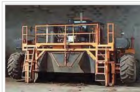
Windrow turner used on maturing piles at a biosolids composting facility in Canada.
